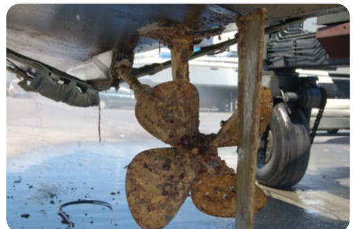
Biofouling on vessel propeller. MPI
