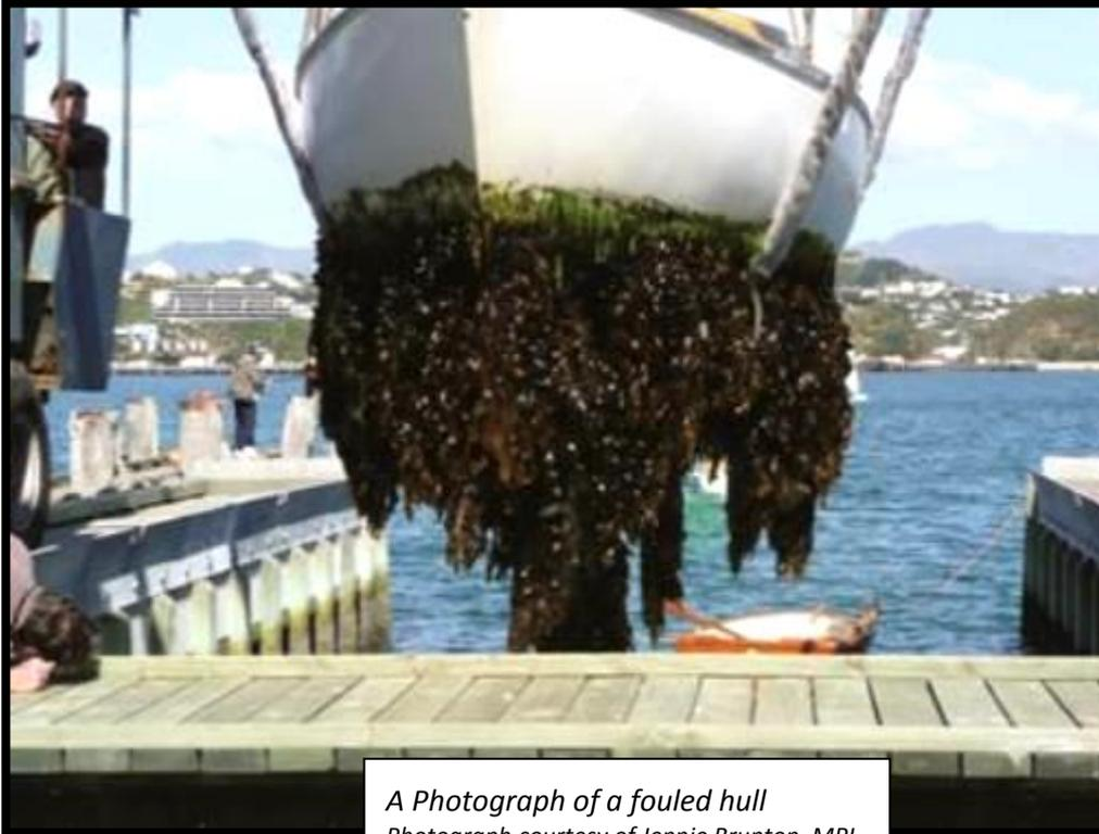
*A Photograph of a fouled hull
