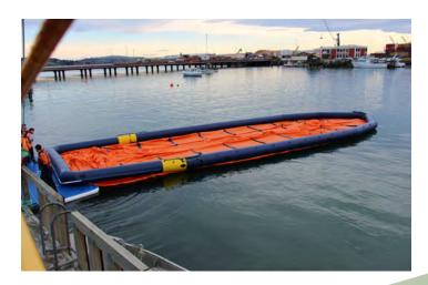
FIGURE 1: NORTHLAND REGIONAL COUNCIL'S FAB DOCK IN USE. ENVIRONMENT SOUTHLAND'S FAB DOCK WILL BE SLIGHTLY LARGER TO ACCOMMODATE THE AVERAGE VESSEL THAT TRAVELS TO THE FIORDLAND MARINE AREA
