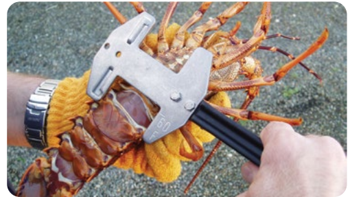
Measuring a female spiny rock lobster (kōura) tail width using a Ministry for Primary Industries gauge. MPI
