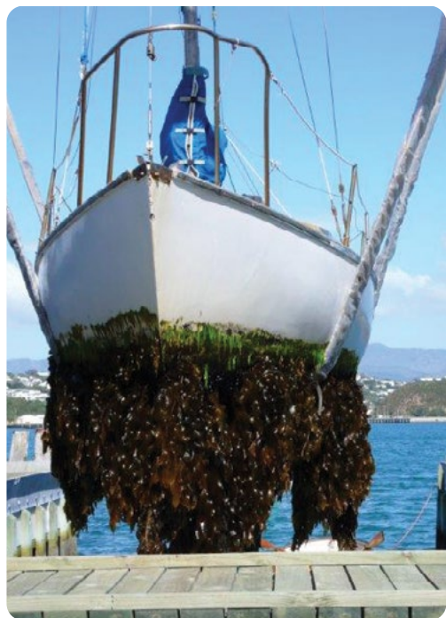
Undaria pinnatifida biofouling on vessel hull. MPI
